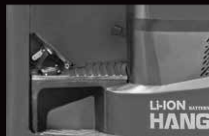
The pedal height can be adjusted electrically
